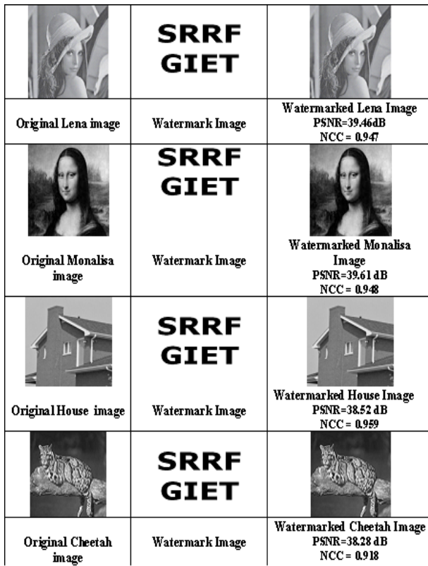
Figure4. Original and Watermarked Images with PSNR and NCC values
